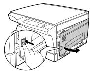
Check the misfeed location. Remove the misfed paper following the instructions for each location in the illustration below.
